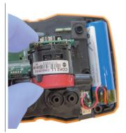
Remove hose connections from the faulty sensor/bridge.
